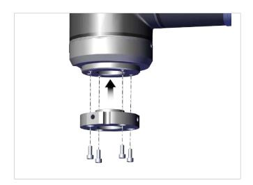
Mount the flange plate on the robot, Tightening torque as specified by the robot manufacturer
