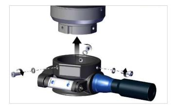
2. Mount the gripper on the flange plate using Nord-Lock washers and machine screws, tightening torque 2 Nm
