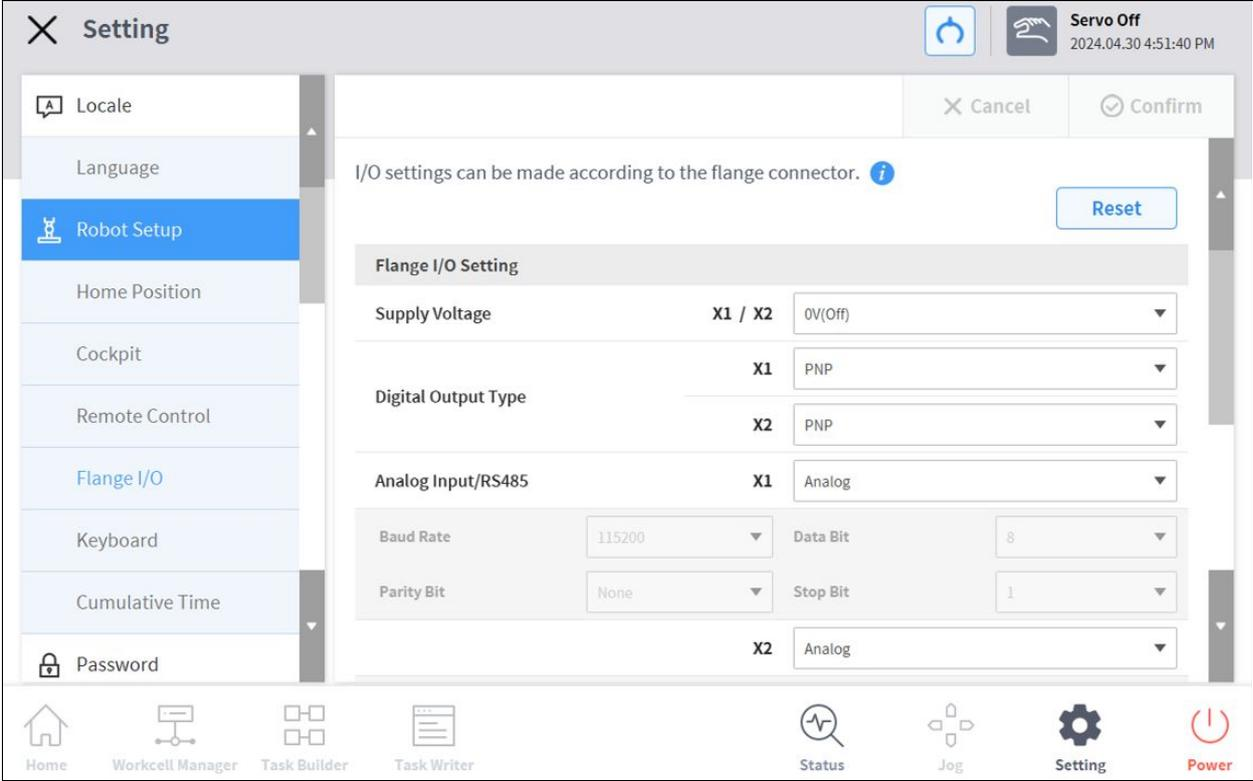
I/O settings can be made according to the flange connector.
