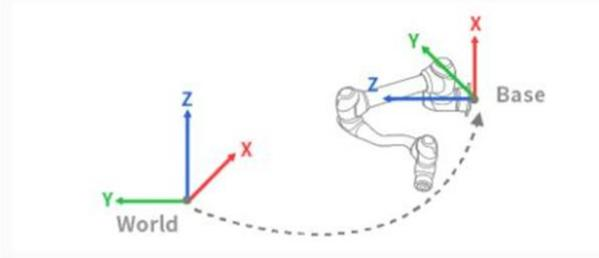
**i** If you change the World to Base relationship, the position of the teaching point relative to the World coordinate system or the User coordinate system based on the World coordinate system in the previously created work file may change. Change is recommended only if the relationship between the actual World coordinate system and the Base coordinate system has changed.
