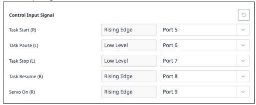
You can assign input ports for Start, Stop, Pause, Resume, and Servo On commands. Press the Reset button to clear the control input signal configuration.
