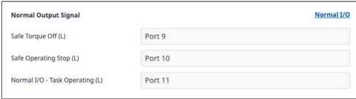
You can assign output ports for STO, SOS, and Task Operating signals.
