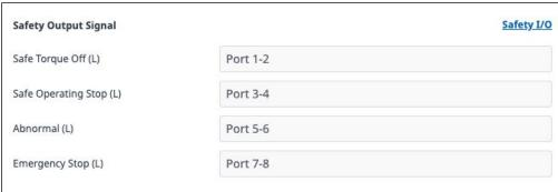
You can assign output ports for STO, SOS, and Emergency Stop signals.
