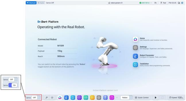
**Servo On** refers to a standby state in which the robot arm can be driven by powering the joint. Servo off when an emergency stop button is pressed or a safety restriction is violated. In the servo off state, the joint is powered off and the robot arm cannot be driven and the **task editor**, **jog plus** associated with the robot arm drive is disabled in the main menu.
